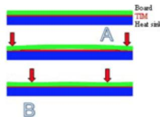
Some PCBs can flex due to the mechanical spacing between the mounting screws and the compression of the thermal interface material between the PCB and the heatsink.
