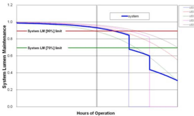
In terms of LED system light output, each LED gradually decreases with time. In the case of a wear-out failure, the light output of the LED which failed goes to zero abruptly. Thus, at the system level, the light output of the LED system drops slightly, depending on how many LEDs are used. At the system level, it is then possible to estimate the time for the system to fall below a desired light output.
