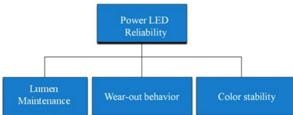
Today, we can develop separate reliability models for LED component lumen maintenance and for LED wear-out failures. In addition, the color stability of light generated by the LED is important for most LED SSL systems.
