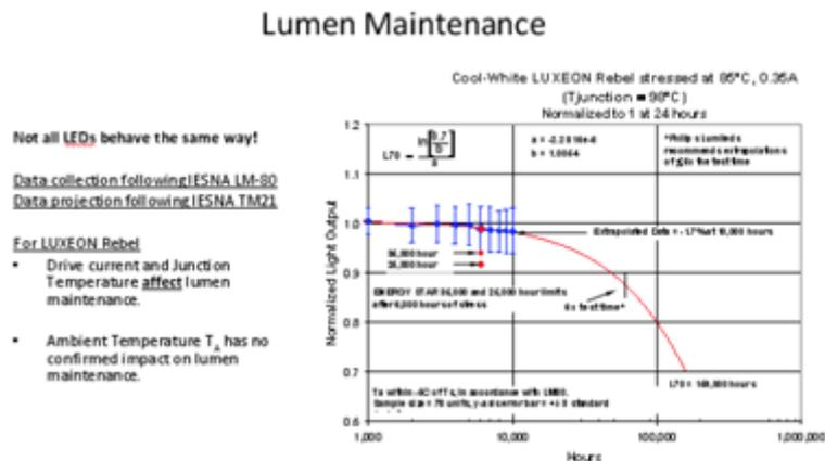
The lumen maintenance graph above shows typical lumen maintenance behavior over time for a Cool-White LED at a specific drive condition. Note that this graph corresponds to 10,000 hours of actual lumen maintenance data. The heavy blue dots
