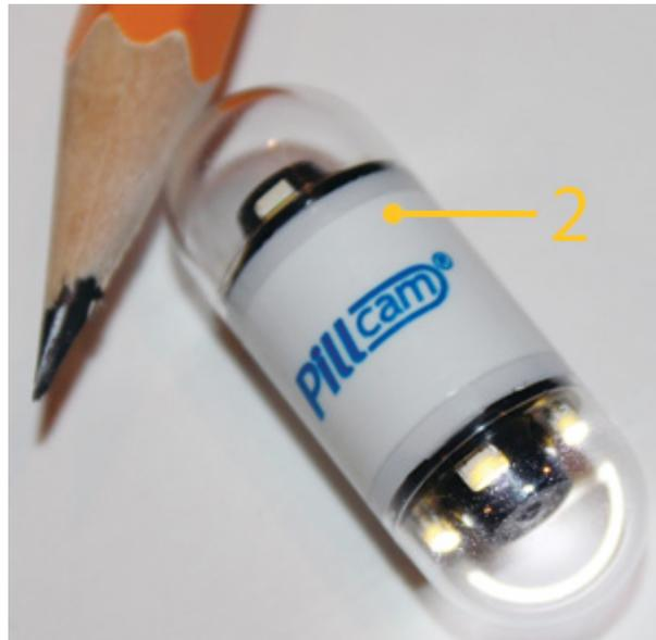
**2. The Pillcam Colon 2 measures 11×26 mm and weighs less than 4g. The four LEDs on each end of the pill flash alternately and allow images to be taken looking forward and behind, deep into the colon mucosa, as the capsule tumbles. There is one Aptina CMOS image sensor at the center of each end of the Pillcam.**
