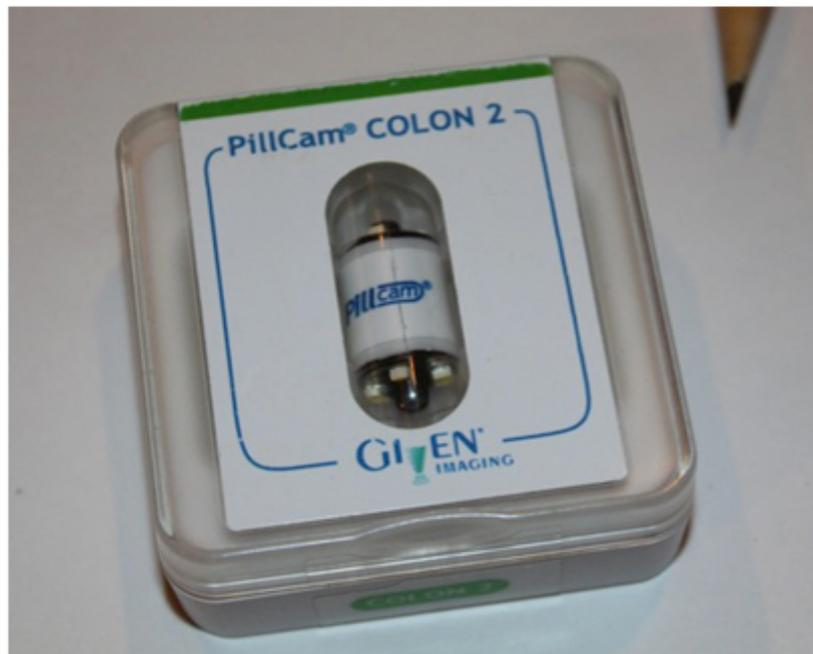
To use the device, the subject swallows the capsule. The images it captures are sent to a sensor array that is worn strapped to the subject's chest and that connects to a data recorder. The subject returns the recorder to the doctor the next day and excretes the use-once Pillcam within a couple of days. (FYI—or perhaps this is TMI—subjects have been known to retrieve and save their capsules for posterity.)
