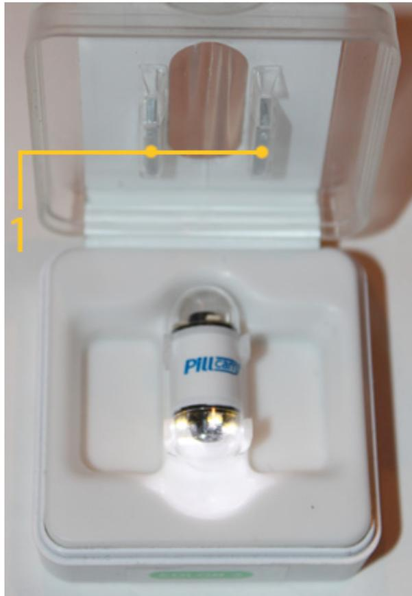
**1. When the unit is closed, two magnetic strips on the lid activate a MEMS switch to keep Pillcam Colon 2 in the off state. The Pillcam activates when the lid is opened.**
