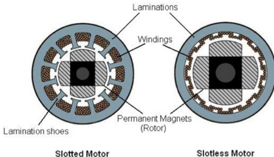
Figure 2: Slotted and slotless motor
