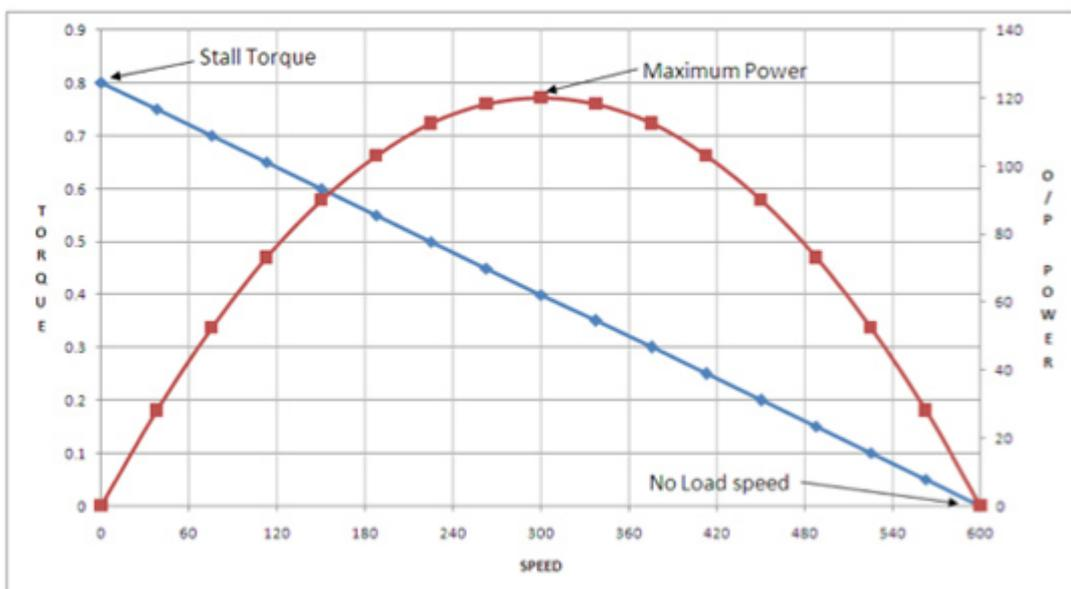
Figure 5: Speed-Torque-Power curve
