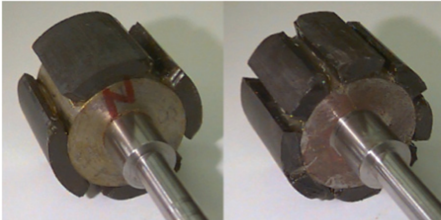
Figure 3: 4 pole and 8 pole – Permanent magnet rotor
