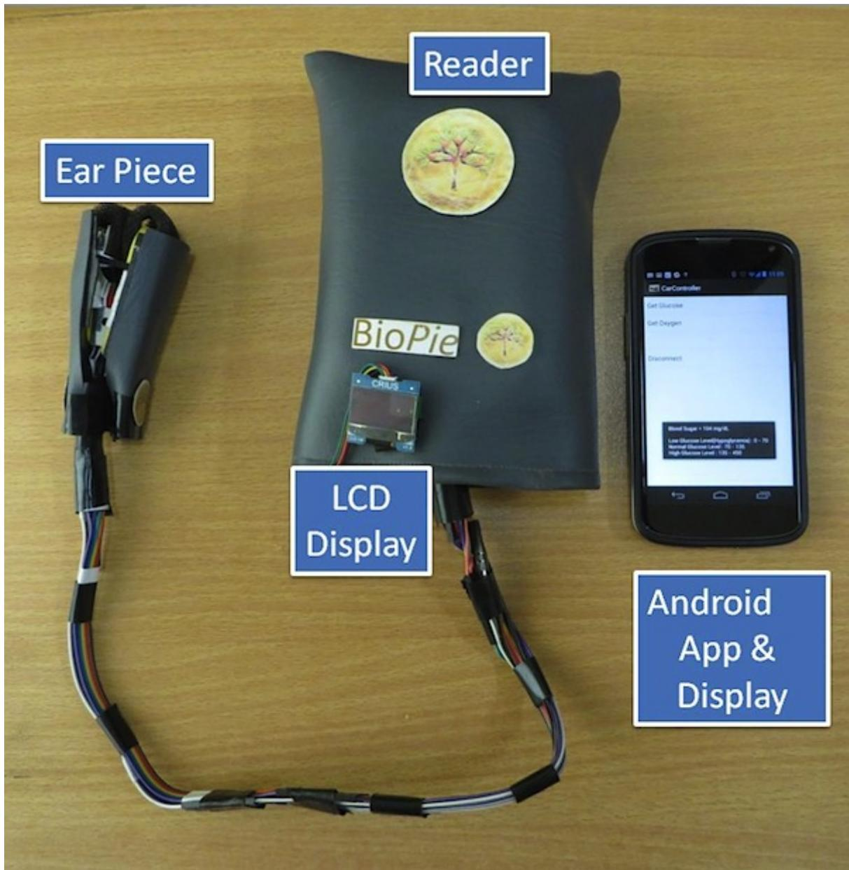
**Figure 5** Complete Setup
