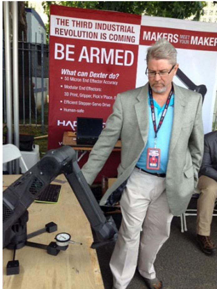
The robot's impressive force feedback, which Gilson demonstrated at World Maker Faire, helps it achieve 50 micron repeatability and feather light touch, making it applicable to tasks including 3D printing, CNC (computer numerical control), and PCBA (printed circuit board assembly). With the right tools and instruction, Dexter could build its own duplicate.
