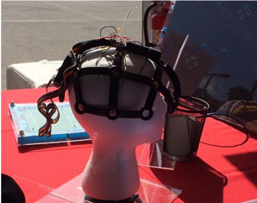
OpenBCI showed off its work at their own World Maker Faire tent, plus got a nod from Microchip, which included the group's device in its tent where the above photo was shot. OpenBCI uses Microchip's ChipKit Arduino-compatible PIC 32 uC, as well as other parts from Texas Instruments (high-powered analog front end) and ST (3 axes accelerometer), among its components.
