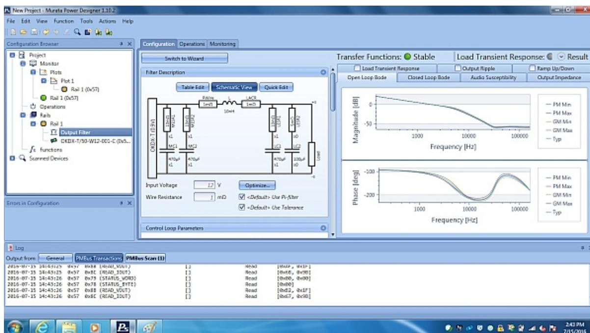
**Figure 3** An example of a digital power graphical user interface. Digital power offers virtually instantaneous control of margining, monitoring operating parameters and configuring the supply.
