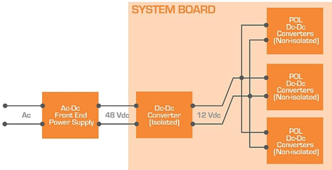
**Figure 1** The proliferation of supply rails at the board level has resulted in an intermediate bus architecture (IBA) that requires multiple POL converters on the system board.
