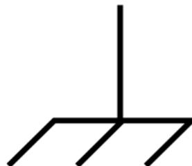
**Figure 3. "Chassis" ground schematic symbol.**
