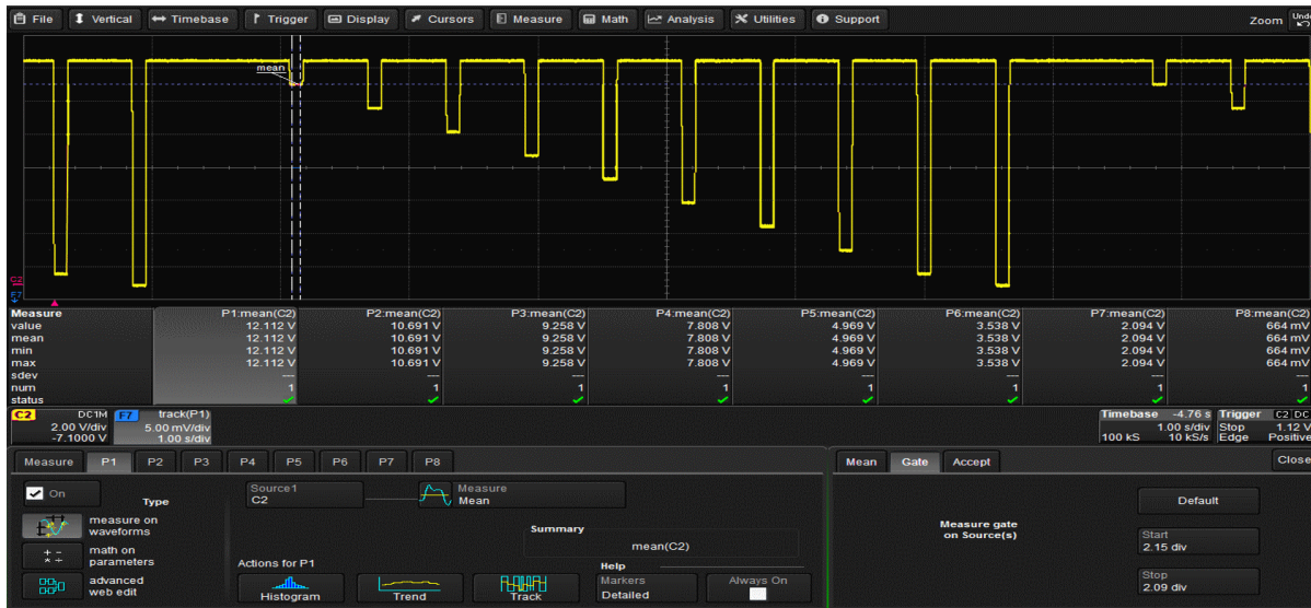
Figure 4. Edge triggering on the lowest dip lets you use multiple mean-voltage measurement parameters.
