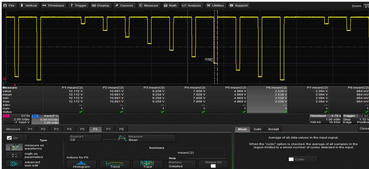
**Figure 5. The oscilloscope simultaneously measures multiple dips while the gated region of the 3.538 V dip is highlighted.**
