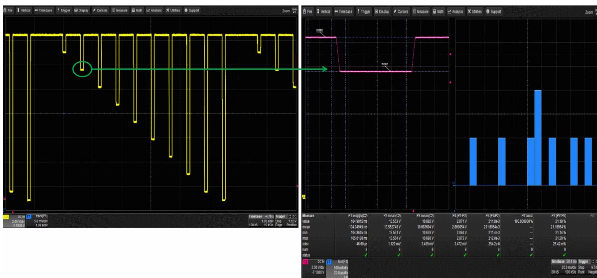
Figure 3. The oscilloscope's runt trigger locks onto second dip and performs the statistical analysis.
