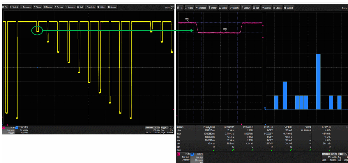
Figure 2. Runt trigger, measurement parameters and histogram quantify the first dip both in terms of voltage and percent.
