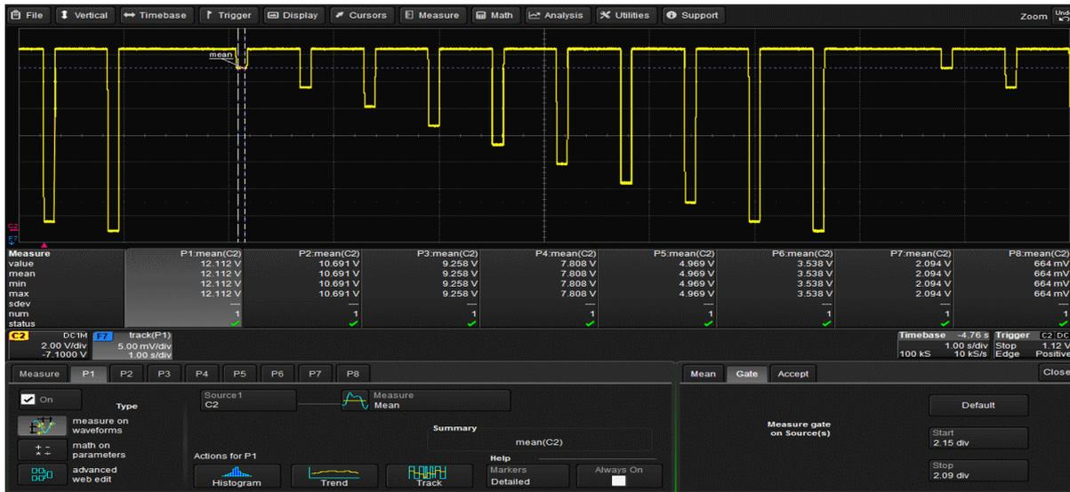
**Figure 4. Edge triggering on the lowest dip lets you use multiple mean-voltage measurement parameters.**
