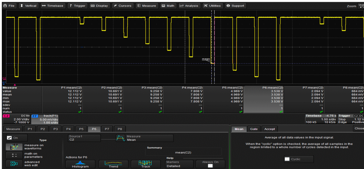
Figure 5. The oscilloscope simultaneously measures multiple dips while the gated region of the 3.538 V dip is highlighted.
