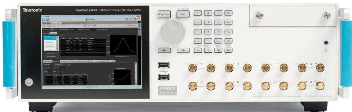
To appreciate the capabilities of the AWG5200, you need to look at its front and rear panels. The front panel has four, eight, or sixteen signal connectors because each channel is a differential output. Standard output voltages are  $\pm 1.5 V_{PK-PK}$  with  $\pm 4 V_{PK-PK}$  optional (see **table** below). There's also a removable hard-disk drive for sensitive applications. It's the rear panel, however, where things get interesting.
