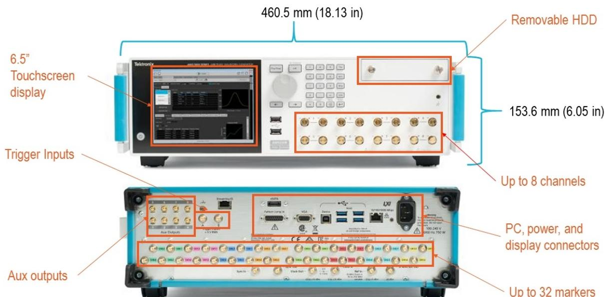
Each channel has four digital "marker" outputs (32 shown for eight channels) that you can use to initiate events based on specified signal conditions. Think of them as trigger outputs. Each channel has an auxiliary output (eight shown) that you can use as a clock signal. Finally, the system has two trigger inputs.
