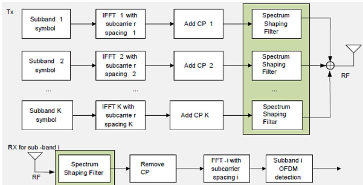
**Figure 3** The adopted waveform for 5G NR (Image courtesy of Huawei)
