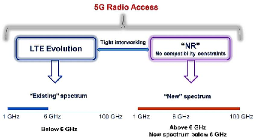
**Figure 1** The 5G Radio Access architecture is composed of LTE Evolution and a New Radio Access Technology (NR) which is not backwards compatible with LTE and is operable from sub-1 GHz to 100 GHz. (Image courtesy of Reference 5)
