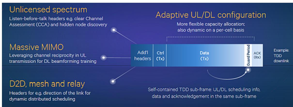
**Figure 4** OFDM's self-contained TDD subframe design is faster and more flexible for TDD switching and turn around than [LTE's 8 HARQ interfaces](#)<sup>3</sup> (Image courtesy of Reference 2)
