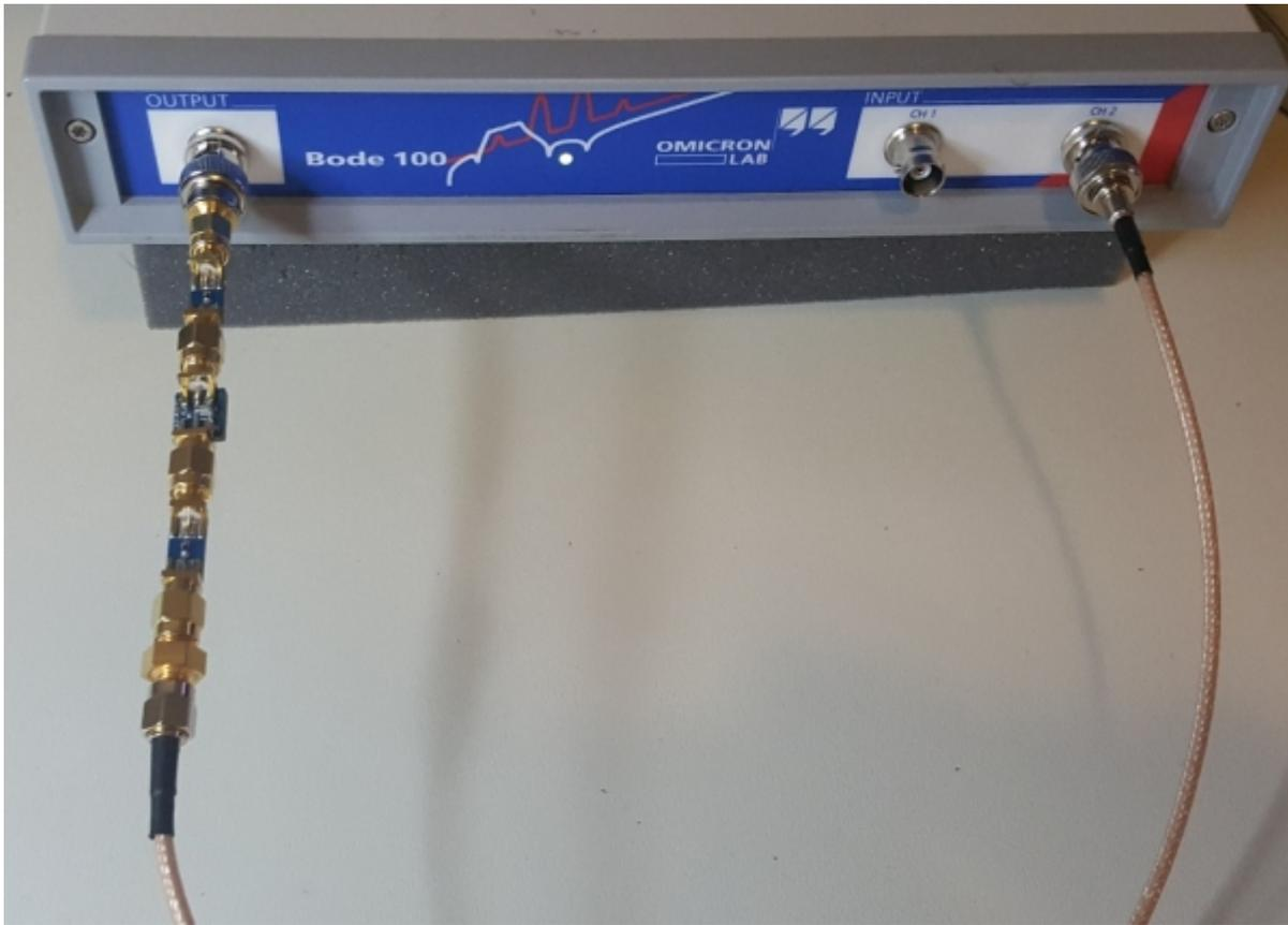
**Figure 4. Two-port impedance measurement with series resistors based on the schematic in Fig. 3**
