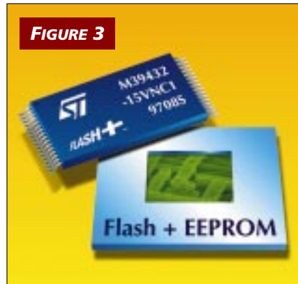
Figure 3 The Flash+ M39432 includes 4 Mbits of flash memory and 256 kbits of parallel EEPROM on one die, operating concurrently at 3.3V and delivering 120-nsec read performance (courtesy SGS-Thomson).
