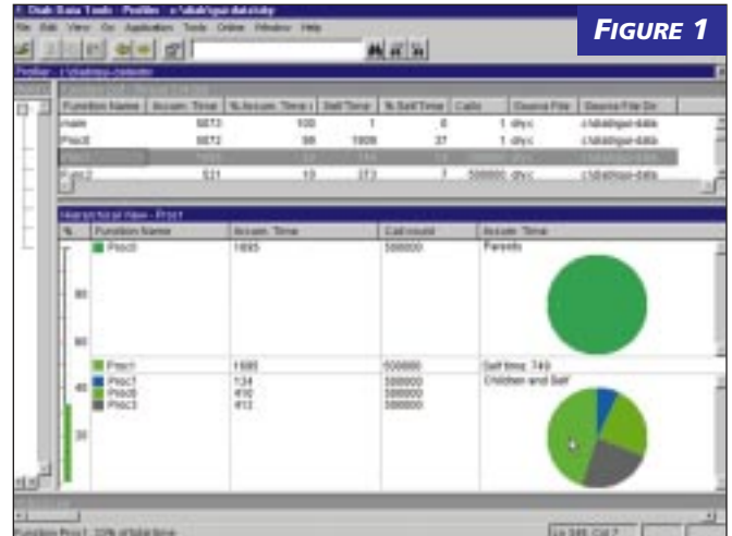
FIGURE 1 VIP examines function-pair relationships at runtime and shows the percentage of time that one function called, or was called by, another.
