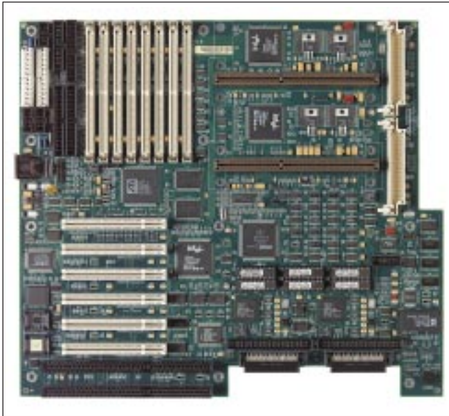
The MegaRUM motherboard from American Megatrends accepts an optional i960 I/O processor that can control dual SCSI channels in an I 2 O implementation.
