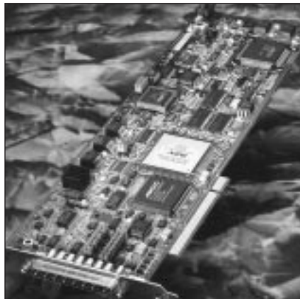
The Hi*Def Accura PCI board from Imagraph not only digitizes analog signals at 140M samples/sec with -500-psec timing accuracy, but also captures high-resolution, noninterlaced images to 1280X1024 pixels at 75 frames/sec.
