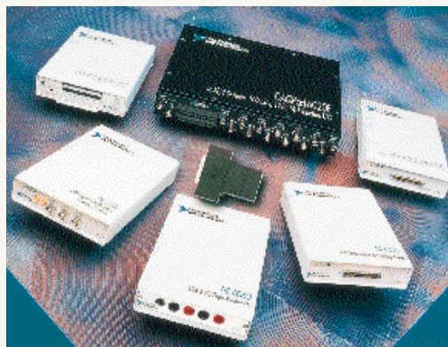
National Instruments offers several USB T&M products. The three units in the foreground are USB instruments. The three units in the back row are USB-based data-acquisition products. In the center is a USB-to-IEEE 488 converter.
