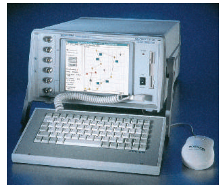
Figure 5: The Noise Com MP2700 wideband multipath fading emulator simulates a long list of fading models on the user-supplied signal.
