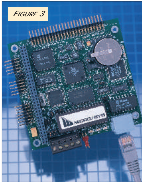
FIGURE 3 The new 3.633.8-in. PC/104 single-board computer from Micro/sys includes an Ethernet port and TCP/IP software preloaded into flash memory.
