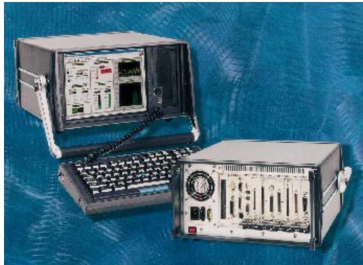
Although it resembles the "lunch-box" PCs of yesteryear, the PXI-1025 Megapac is much smaller. The unit lets you swap the CPU, the power supply, and the CompactPCI modules without removing any covers.
