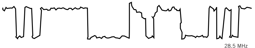
In the example in the text, you want to preserve the 4-nsec rise time in this video signal; the corner frequency of your filter is thus 0.35 \div 4 nsec, or 87.5 MHz.
