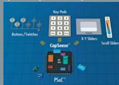
A single mixed-signal programmable device can sense up to 48 lines.
