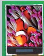
The SSD1784 display controller can support 132×60-pixel resolution CSTN LCDs and achieve 65,000 color combinations in a simple application circuit requiring a microcontroller.
