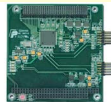
The four-port USB104+ PC/104-Plus USB 2.0 host controller delivers high current drive and can power external USB mass-storage devices.
