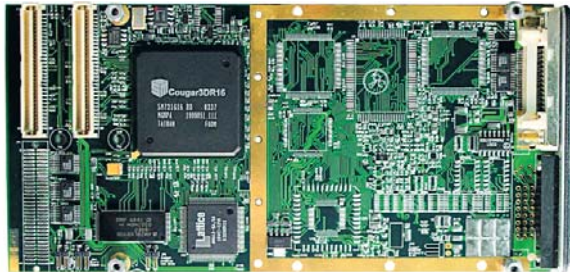
The Topaz/PMC card combines VGA/LVDS/DVI graphics with video, DVI, and RGB digitizers.
