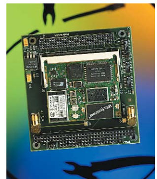
The PC/104-Plus PPM-Wireless module from WinSystems delivers 802.11b/g wireless-Ethernet connectivity for industrial applications.
