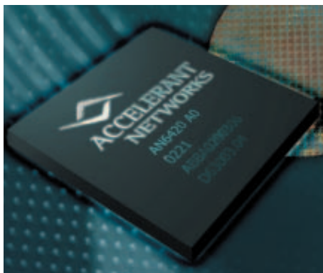
The AN6420 quad backplane transceiver consumes 0.2W per 10-Gbps channel across 20 in. of FR4 and two backplane connectors with a maximum range of 60 in., all with 0% effective overhead.
