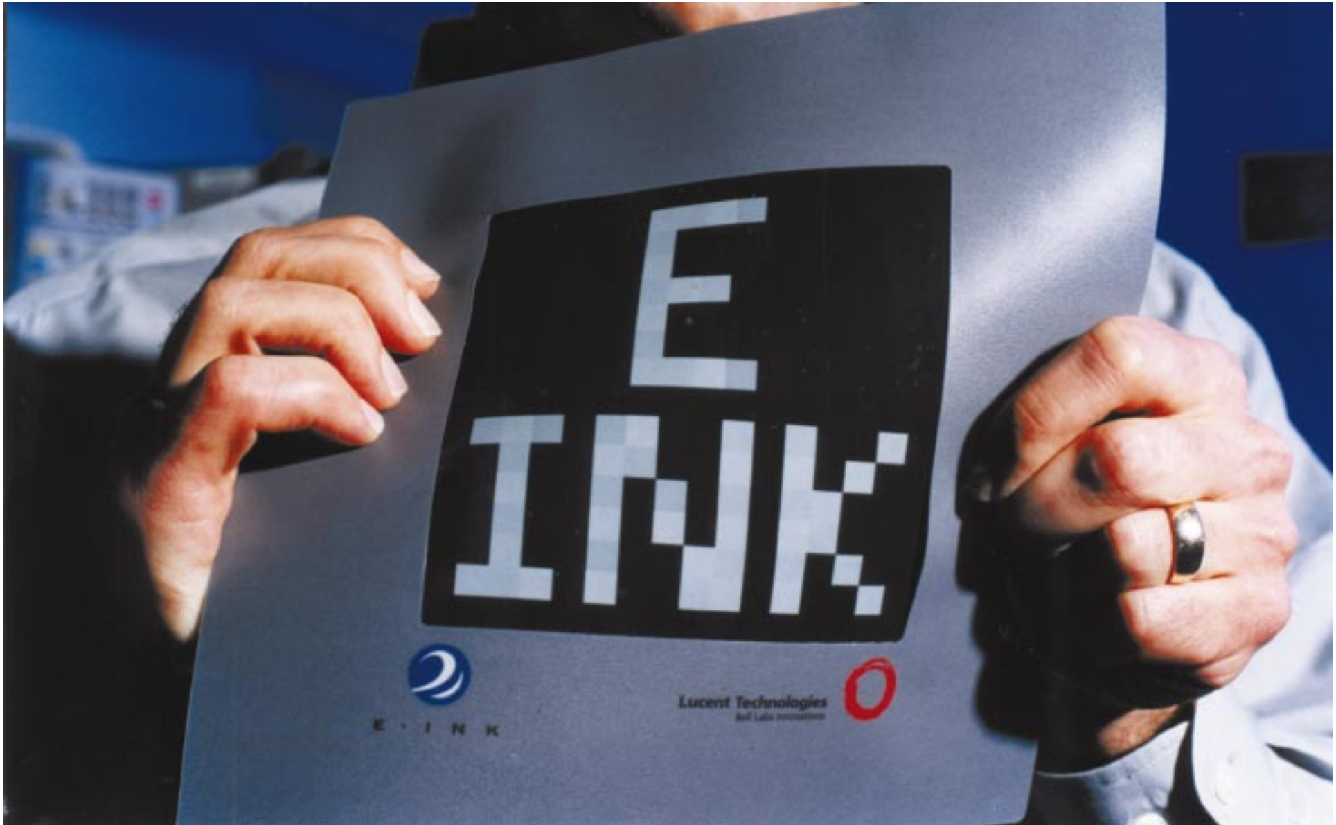
A 5×5-in. prototype of a flexible, active matrix addresses an electronic-ink display (courtesy E Ink Corp).
