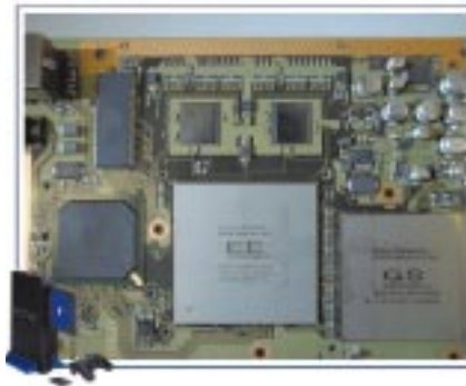
Figure 2 PlayStation 2 uses custom-packaged DRDRAMs to reduce memory and system-board cost.
