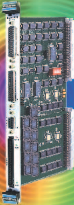
The Model 6802 6U VME board from Pentek offers 32 channels of 24-bit delta-sigma analog-to-digital conversion and a front-panel-data-port output interface for high-speed data transfers.
