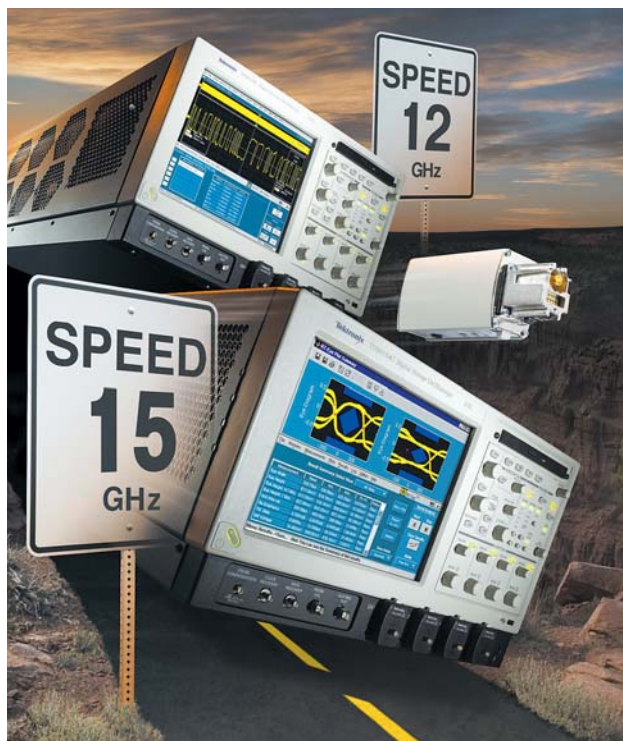
The TDS6124C (top) provides 12-GHz, real-time bandwidth and is upgradeable to become a TDS6154C, which offers DSP-extended, 15-GHz, real-time bandwidth. The P7313 Z-active differential probe (amplifier module is at the right) provides a high dc input impedance but offers the stable high-frequency loading usually associated only with low-impedance Z_0 probes.
