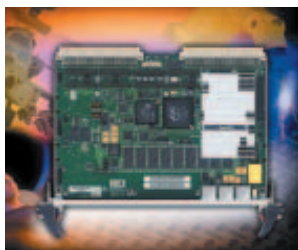
A new single-board computer from Motorola Computer Group boosts data transfers across the VMEbus backplane to 320 Mbytes/sec.
