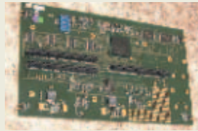
Figure A The initial TriCore board occupies as much area as possible and includes a prototyping area for those afterthought-engineering exercises.
