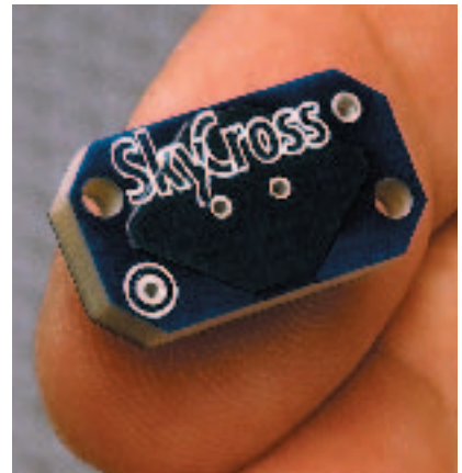
SkyCross antennas, such as this 5.25-GHz antenna for wireless-LAN applications, use meander-line technology, folding lines in a zigzag form, for compactness. The folded structures couple electrically to enhance performance.
