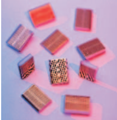
A frequency-selective surface, created by printing patterns of inductors and capacitors on film, is the basis for these 9×13×2.2-mm ClearLink antennas from e-tenna, which work for 2.4-GHz Bluetooth and 802.11b applications.
