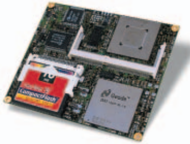
Figure 3 The ETX (Embedded Technology eXtended) form factor from Jumpetec supports both the ISA and the PCI buses and all I/O signals through four 100-pin connectors.
