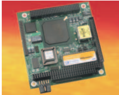
Figure 2 PC/104 computer modules, such as this Bobcat board from VersaLogic, make effective off-the-shelf, plug-in processors for embedded devices.
