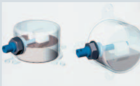
A clever liquid-level sensor adjusts to tilt of the vessel you are measuring by using a cylindrical float with an integral magnet. The float rotates as it senses a liquid level above threshold (left) and below threshold (right).
