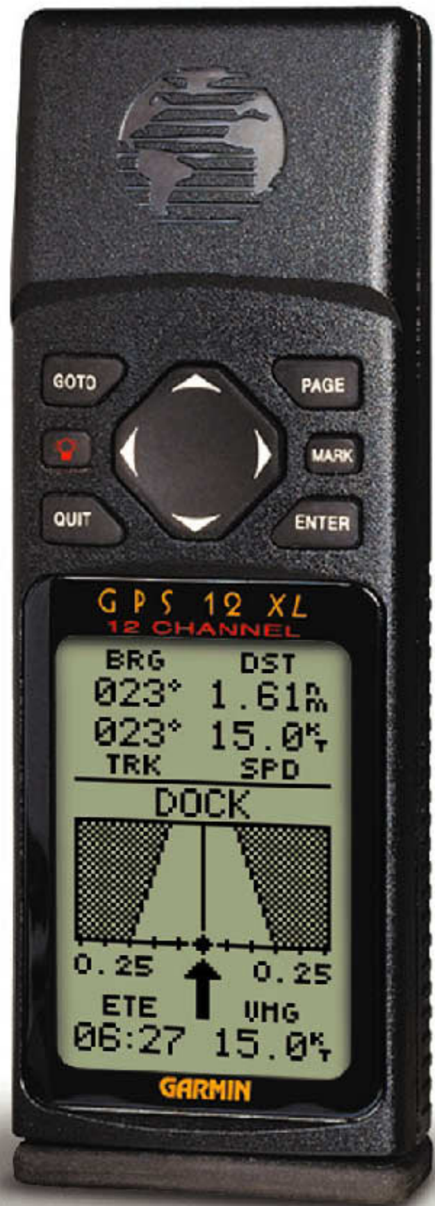
Garmin's GPS12XL demonstrates the ergonomics of giving the antenna the best possible view of the sky.
