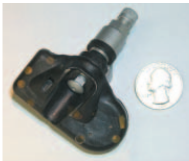
TRW's valve-mounted sensor package measures a little over an inch in length.
