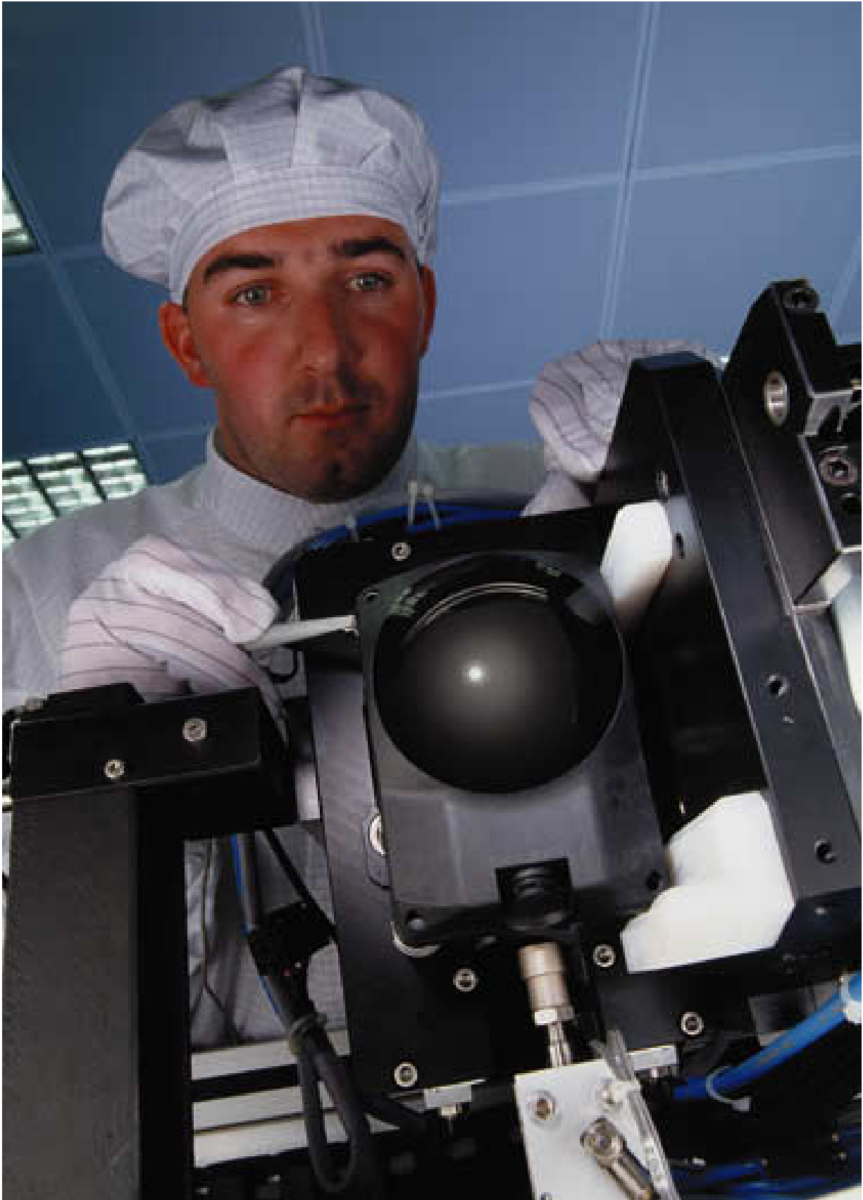
ACC radars, such as this 77-GHz example, mount a single module in the vehicle's front bumper (courtesy Robert Bosch).
