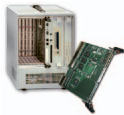
Figure 4 Aurora Technologies' StarFabric development kit integrates the CP-SFX8 fabric card with an eight-slot, PICMG 2.17-compliant backplane and a portable aluminum enclosure.
