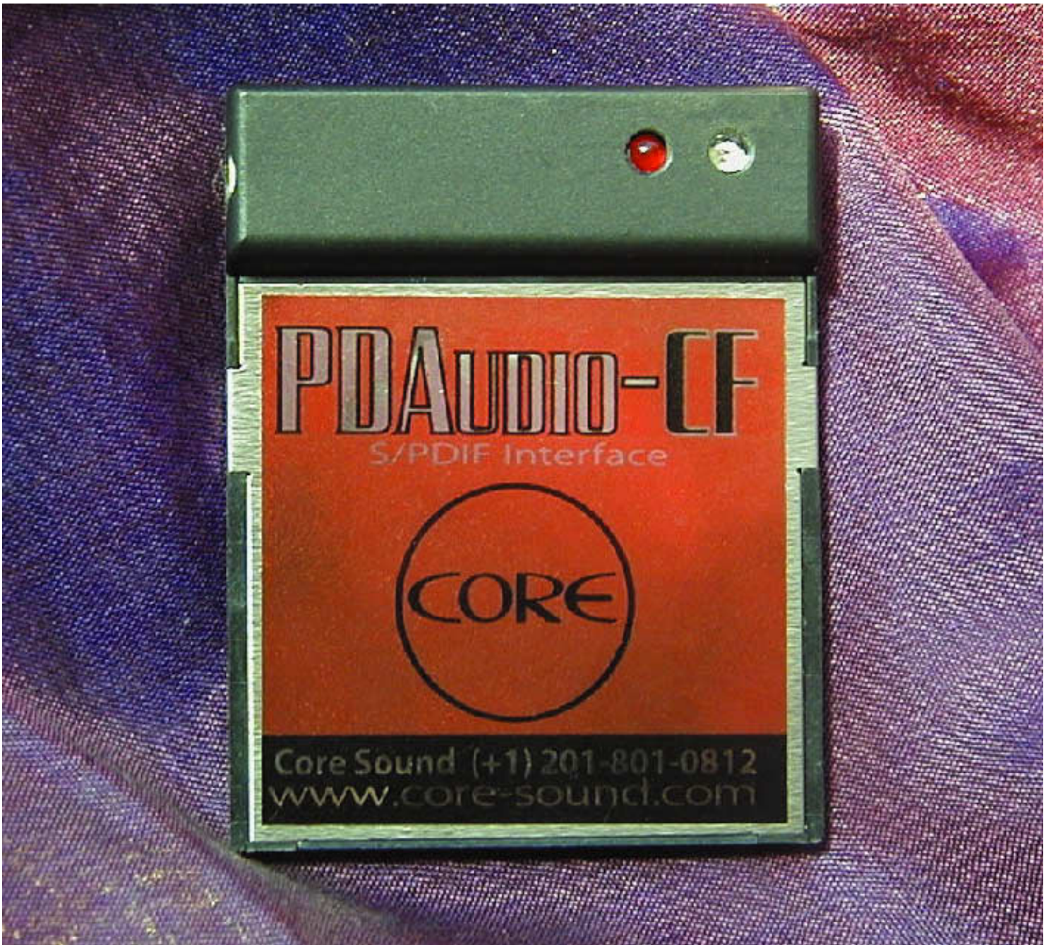
The PDAudio-CF digital sound card is the centerpiece of the PDAudio system (courtesy Core Sound).
