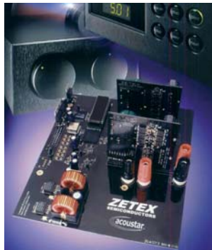
Evaluation versions of the Class-Z amplifier are built in discrete form - an integrated controller chip will follow.
