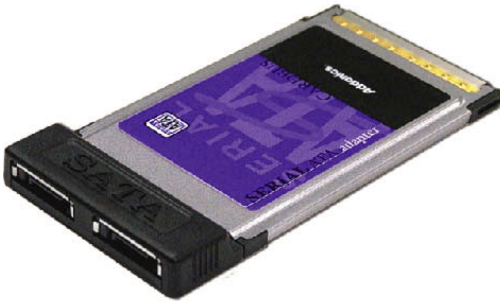
Abit's adapter turns any ATA or ATAPI peripheral into a Serial ATA equivalent (top), and Addonics Technologies' adapter enables you to use Serial ATA peripherals with systems containing CardBus slots (bottom).
