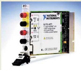
The isolated-input, 7½-digit PXI-4071 DMM (dc/true-rms-ac, V/I/Ω) and high-speed digitizer in PXI format takes seven dc readings/sec at full resolution and 10k samples/sec at 4½-digit resolution. The module also operates as an isolated digitizer with a maximum acquisition rate of 1.8M samples/sec and a maximum resolution of 23 bits.
