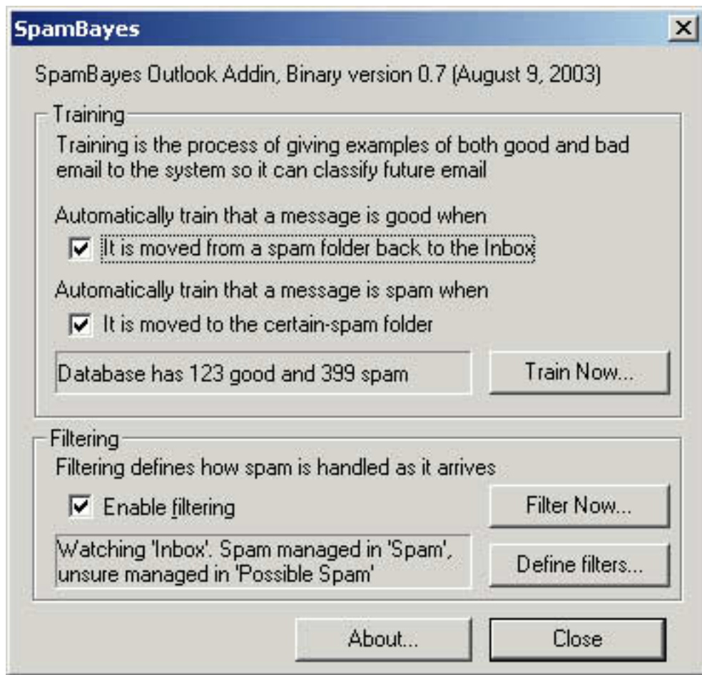
Figure 1 SpamBayes can run either stand-alone or as a plug-in integrated within Outlook (a). You can customize its responses when incoming e-mail arrives, as well as the probability scores that determine whether each message is "ham," potential spam, or spam (b).
