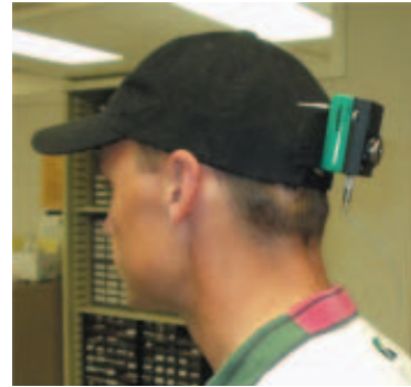
Figure 5 An early prototype that mounted on the back of the golfer's head still had the accelerometer axis parallel with the spine.
