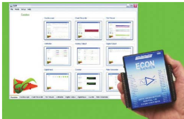
The instrumentlike Go! software that accompanies the Econseries USB-connected data-acquisition modules enables the modules to perform a variety of functions without programming.
