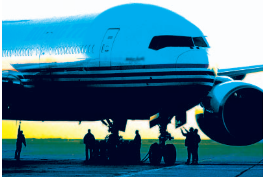
Figure 1 The Airplane Health Management program extensively monitors the aircraft in flight and, while in flight, relays information to ground personnel, so necessary maintenance work can start as soon as the plane stops (courtesy Boeing Commercial Airplanes).
