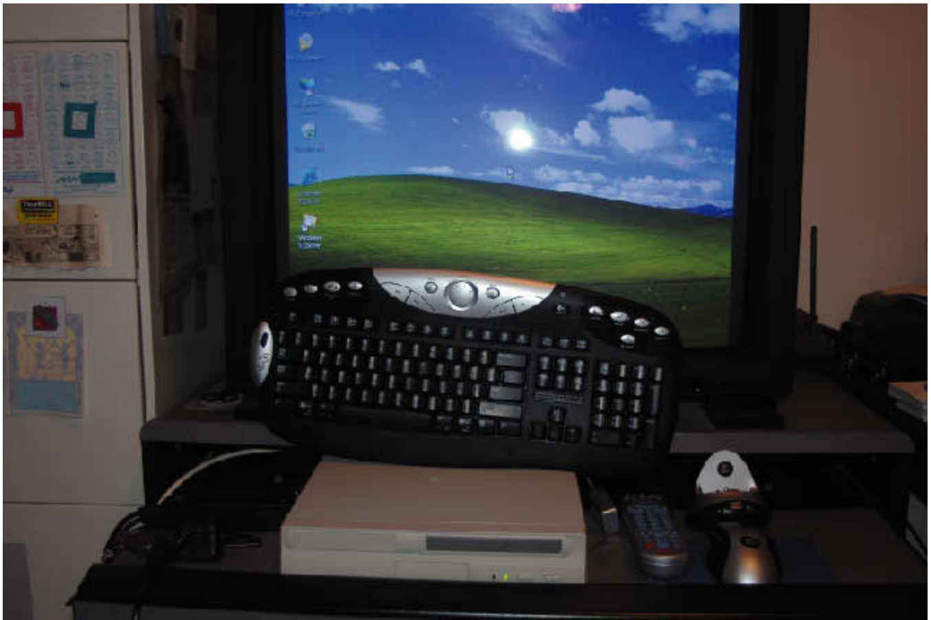
The RF-based wireless keyboard, mouse, and remote control worked just to the desired 10-foot distance.
