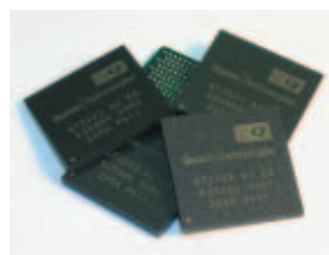
The M69850AWG from Mitsubishi for 10-Gigabit modules consumes only 1.2W of power (left). The QT2022 10-Gbps PHY device from Quake consumes less than 900 mW (right).
