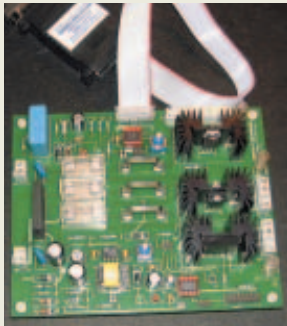
Figure A Ensure that your test board includes safety features, such as fuses, indicators, and easily accessible test points.
