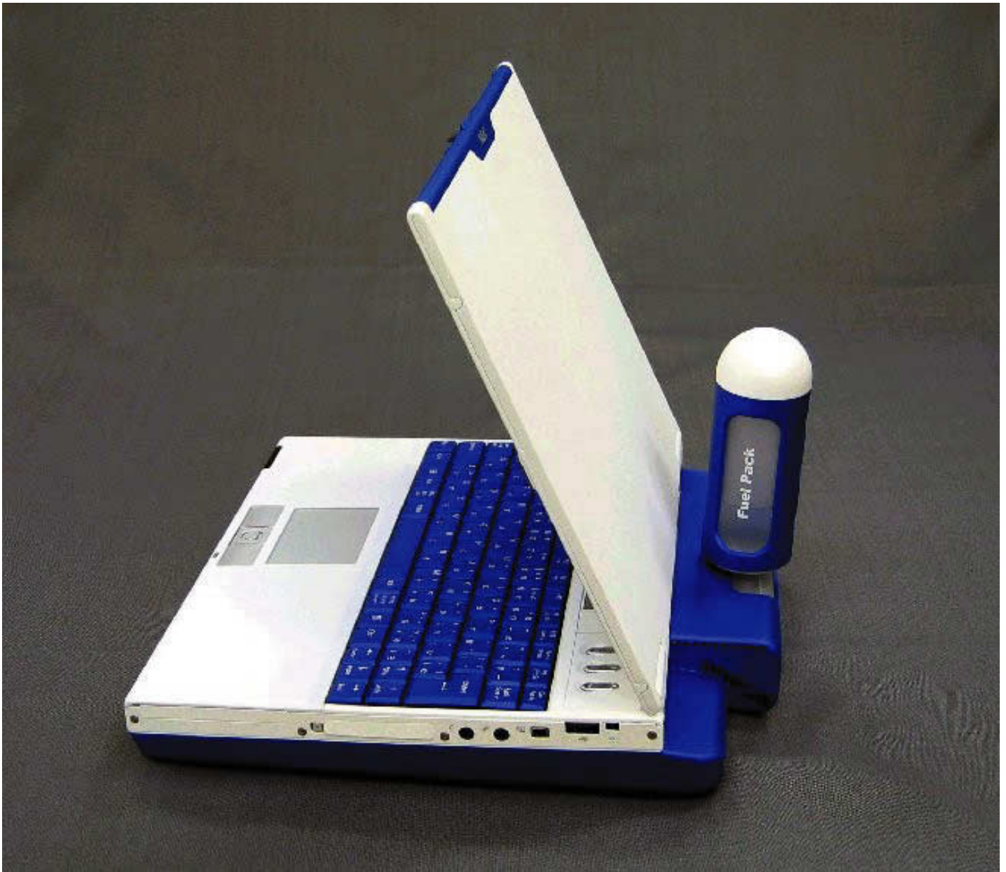
This proof-of-concept model of a fuel-cell-powered notebook PC from NEC uses bottles, as opposed to plug-in cartridges, to supply the methanol fuel.
