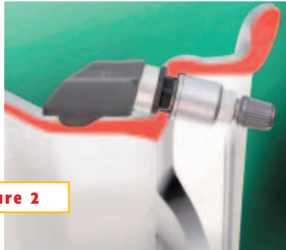
Beru's sensor module mounts inside the tyre on the valve stem.
